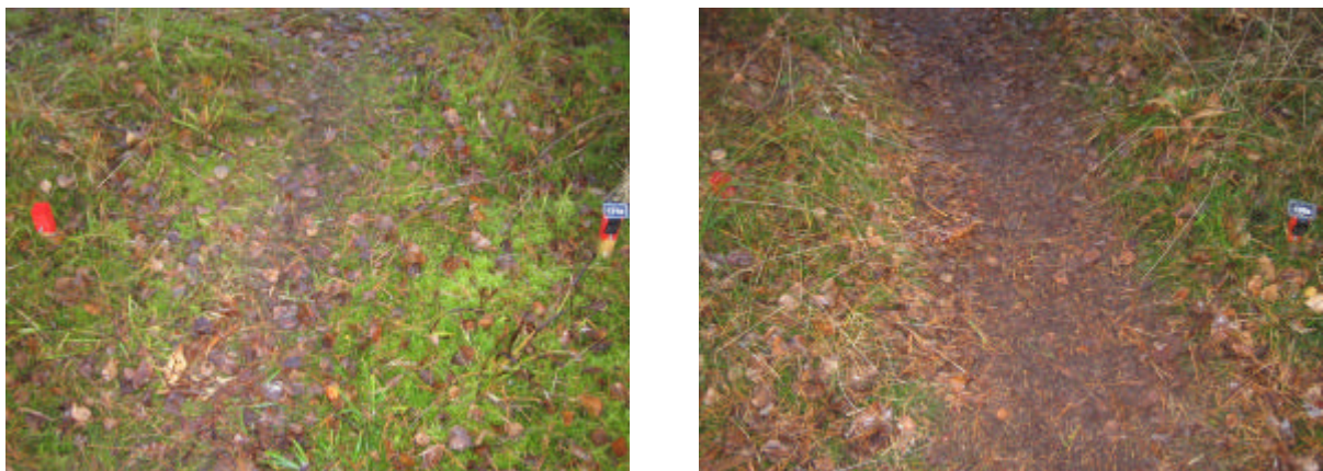
Figure 2: Example of pictures from the database. Both are from the site in Tisvilde Hegn (Sandy soil/pine forest). Both are taken the November 26 2005. Both are from the mountain bike tracks. To the left the track issued to 7 passages per 14 days (a total of 133 since the start of the experiment). To the right the track issued to 105 passages per 14 days (a total of 1995 passages).
